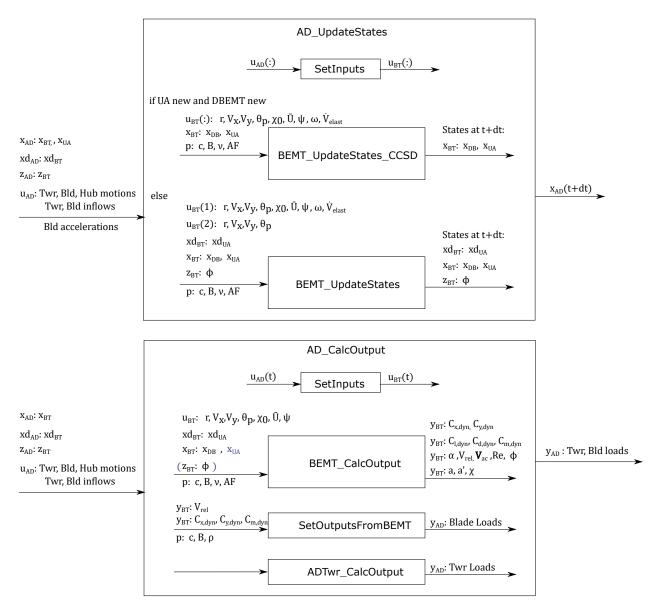
Figure 6: Scheme of AeroDyn states and output routines
