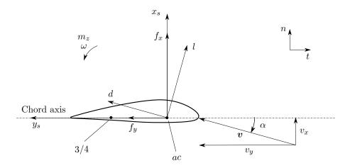
Figure 1: OpenFAST coordinate system for a blade cross section
