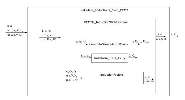
Figure 8: Scheme of main subroutines used in BEMT
