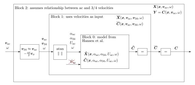
Figure 2: Inputs and outputs for different "blocks", where block 0 is the model from Hansen et al. [1], and block 2 represents the OpenFAST dynamics stall module.
