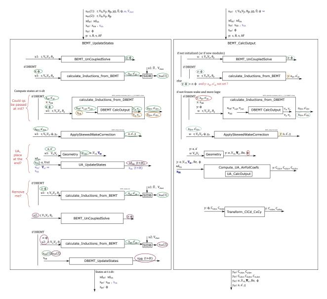
Figure 7: Scheme of BEMT update states and output routines
