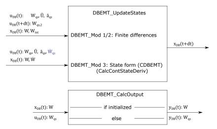
Figure 3: Scheme of DBEMT. The option DBEMT\_Mod=3 is added
