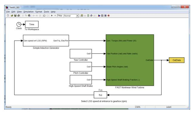
Figure 13: Test01\_SIG.mdl Sample Model for Simulink
