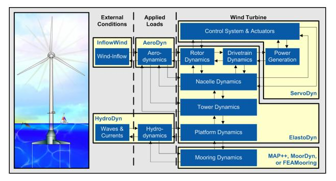
Figure 3: FAST control volumes for floating systems (BeamDyn and OrcaFlexInterface not shown)
