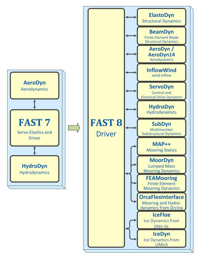
Figure 1: Architectural comparison of FAST 7 and FAST 8
