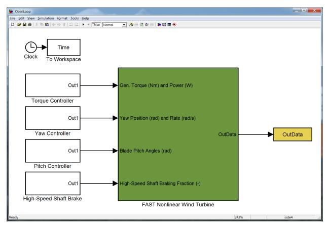
Figure 12: OpenLoop.mdl Sample Model for Simulink
