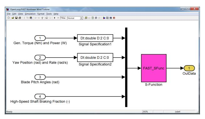
Figure 11: FAST v8 Nonlinear Wind Turbine Block in Simulink
