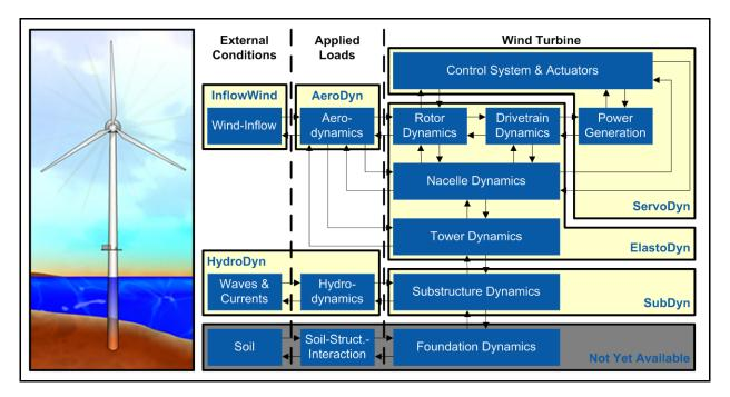
Figure 2: FAST control volumes for fixed-bottom systems (BeamDyn, IceFloe, and IceDyn not shown)
