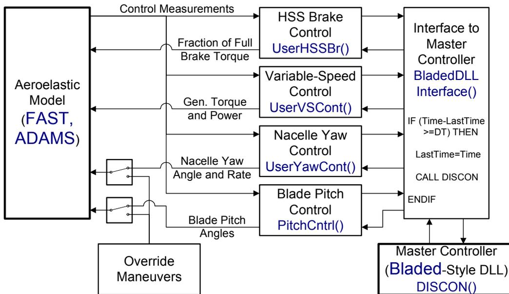
**Figure 25. Interface to a Bladed-Style Master Controller DLL.**
