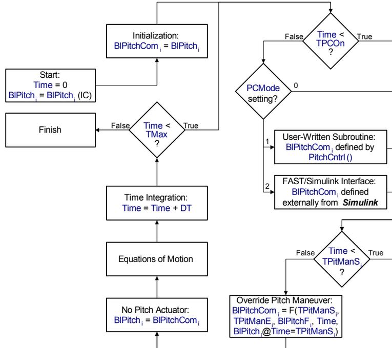
Figure 21. Flowchart of Blade Pitch Control Runtime Options.
