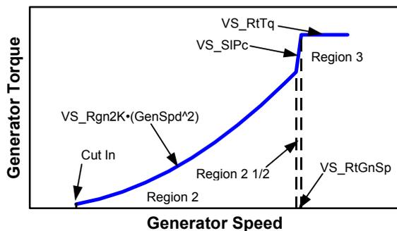
Figure 22. Torque/speed curve for simple variable-speed control.
