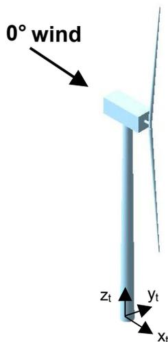
**Figure 3. Tower-base coordinate system.**
