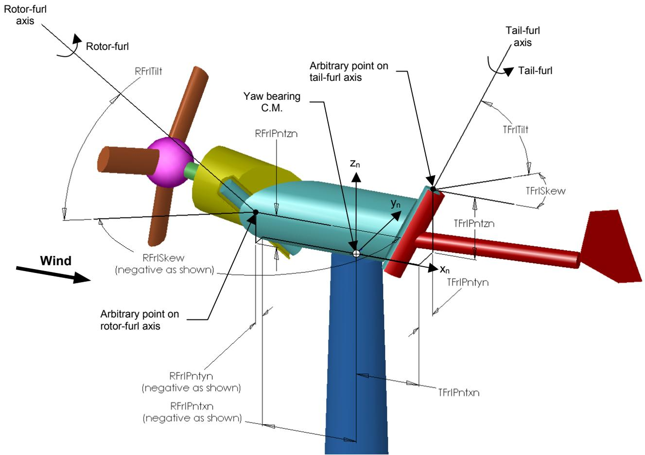
Figure 17. Layout of a three-bladed, upwind, furling turbine: furl axes.
