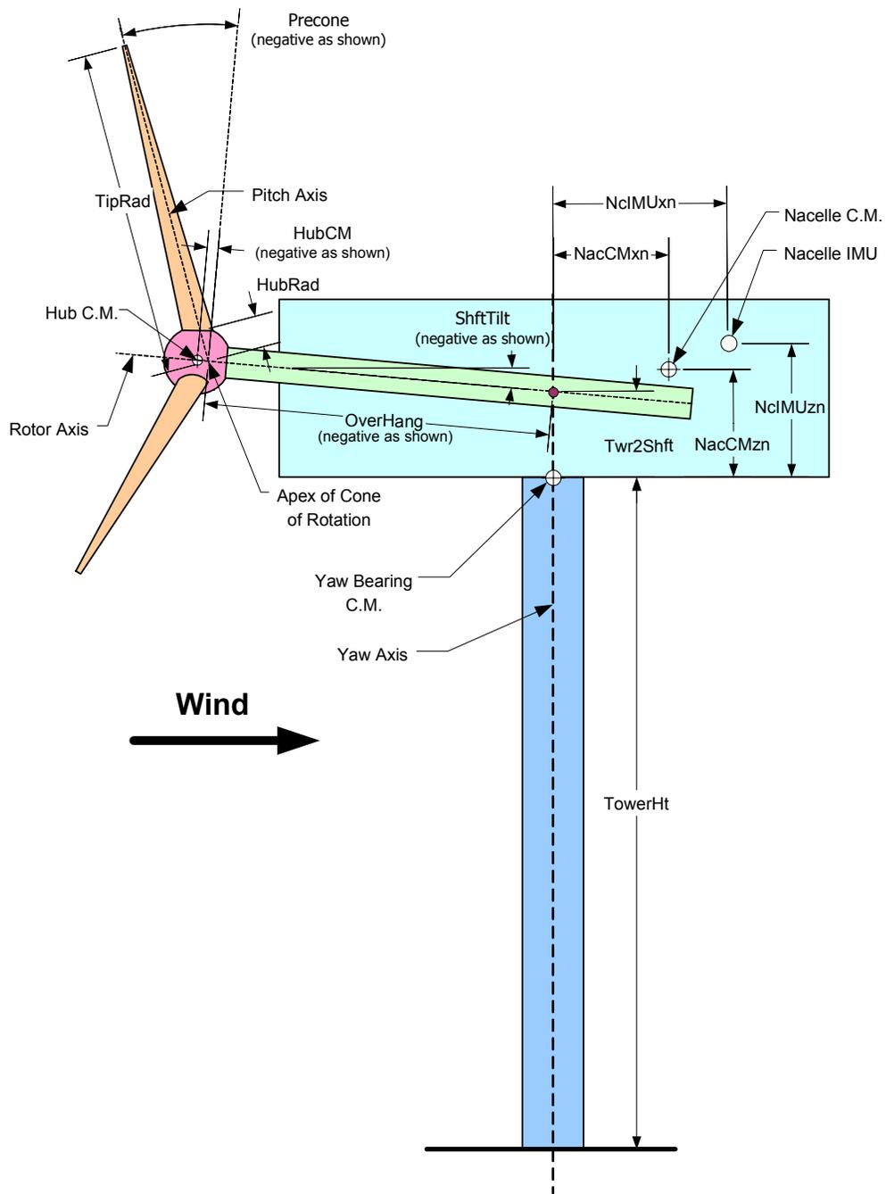
Figure 16. Layout of a conventional, upwind, three-bladed turbine.
