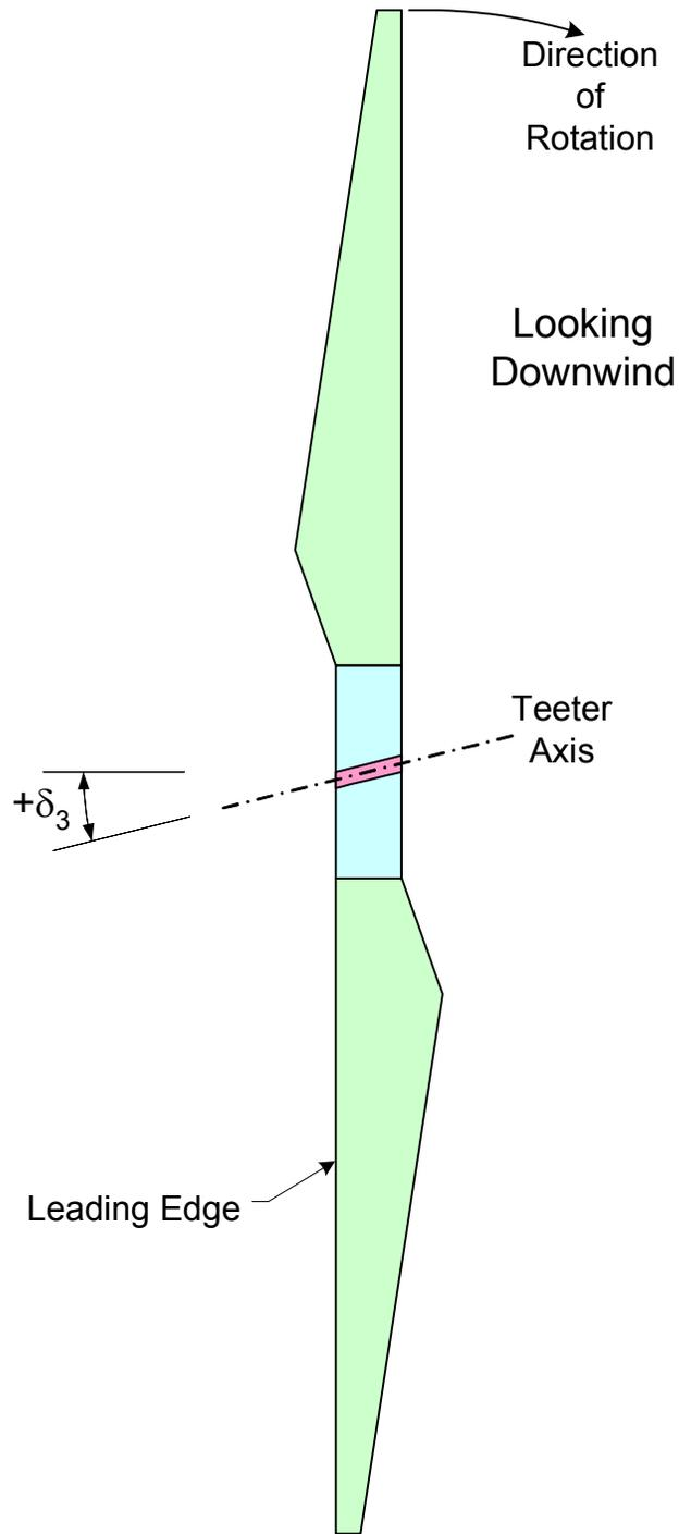
Figure 15. Layout of a two-bladed rotor illustrating  $\delta_3$ .
