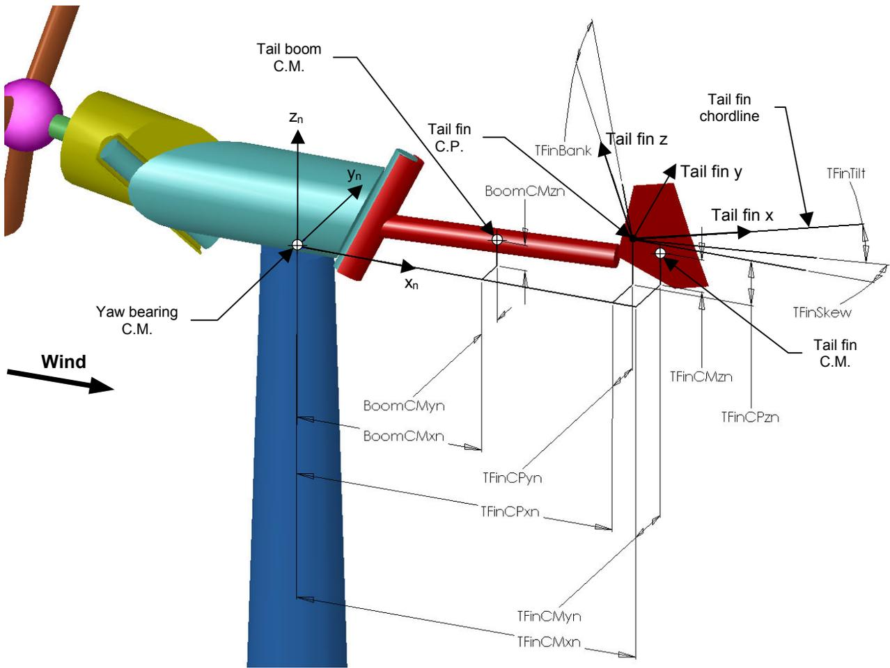
Figure 19. Layout of a three-bladed, upwind, furling turbine: tail-furl structure.
