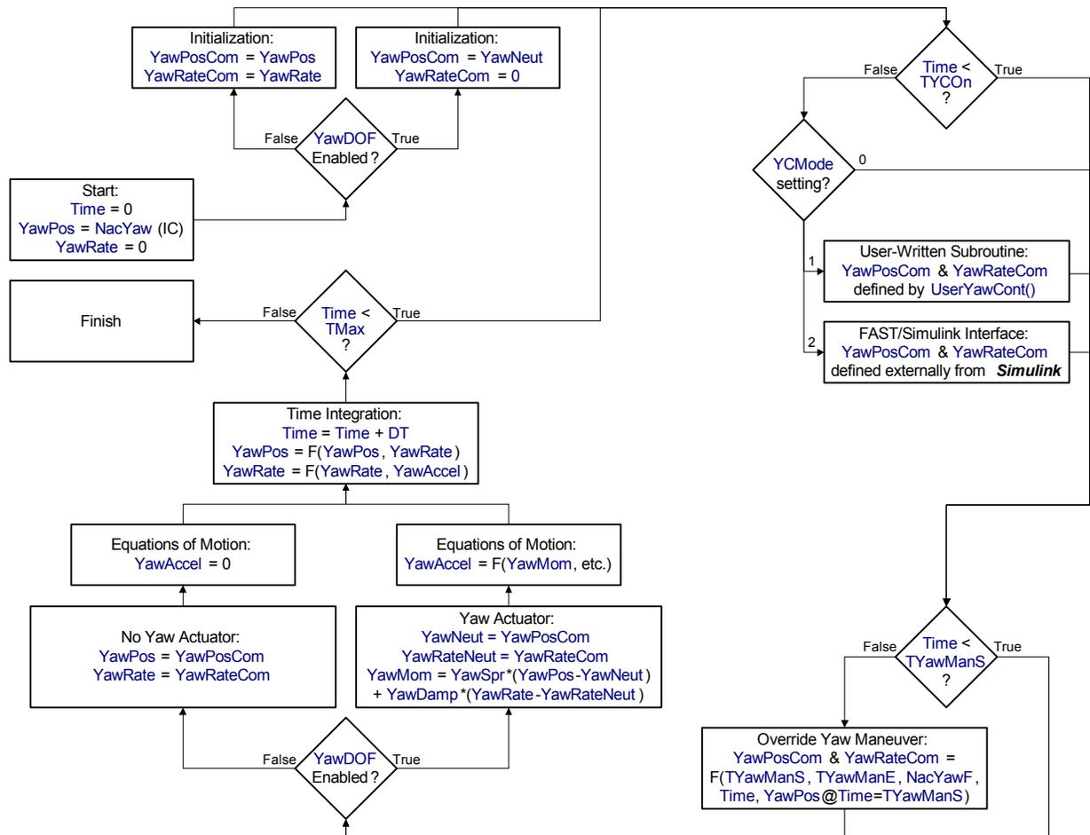
Figure 24. Flowchart of Nacelle Yaw Control Runtime Options.
